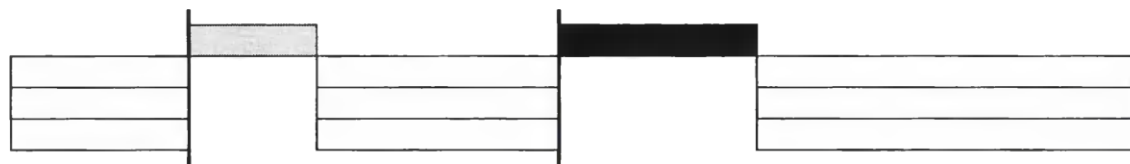
(b) Stop-the-world collection on multiprocessor, single collector thread
